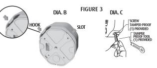
VIEW SHOWING HOW TO FIX THE COVER TO THE BASE
