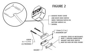
VIEW SHOWING MAGNET INSTALLATION NB: FITTING UNIT AWAY FROM DOOR (OPTIONAL)
